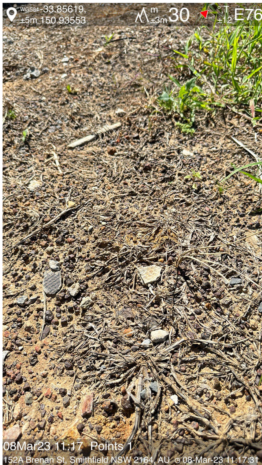
Plate 50: Example of potential ACM observed on the surface of 152a Brennan Street.
