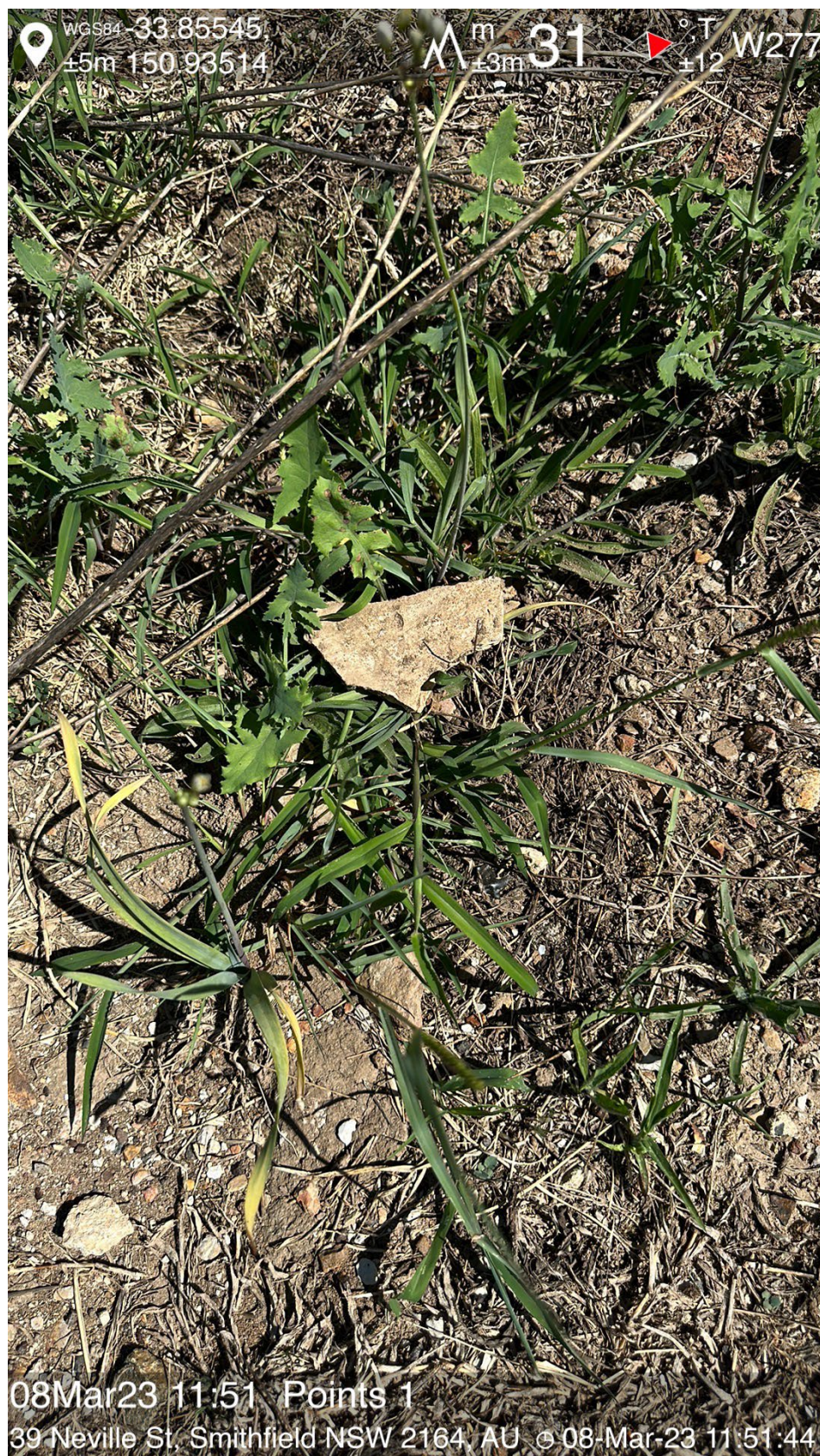
Plate 23: Example of potential ACM observed on the surface in this part of the site.
